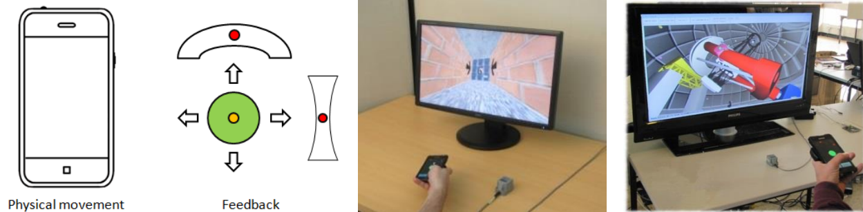
Figure 1. Smartphone-Based interaction techniques to navigate into a 3D museum exhibit: a) principle of use, b) controlled experiment, c) integration in an in-situ exhibit.
