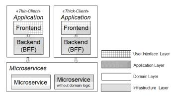
Figure 1. Software building blocks and their layers in a microservice-based application
