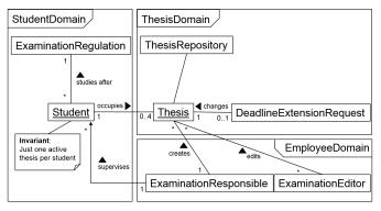
Figure 8. Thesis specific piece of the domain model including DDD patterns
