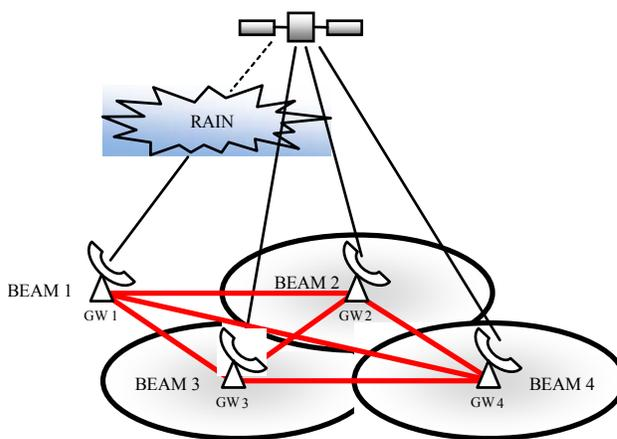
Figure 4. Smart Gateway Concept
