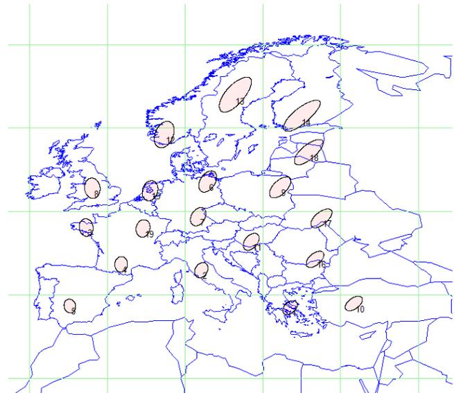
Figure 3. Representative dual polarised 19 beam Gateway configuration over Europe
