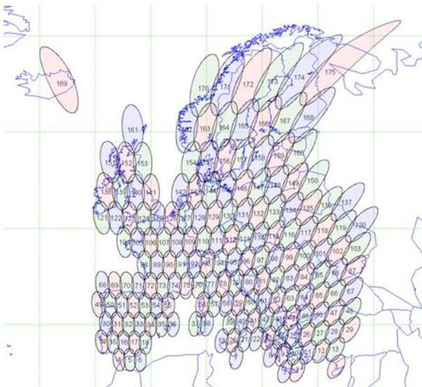
Figure 1. Representative 175 single polarised user beams over Europe
