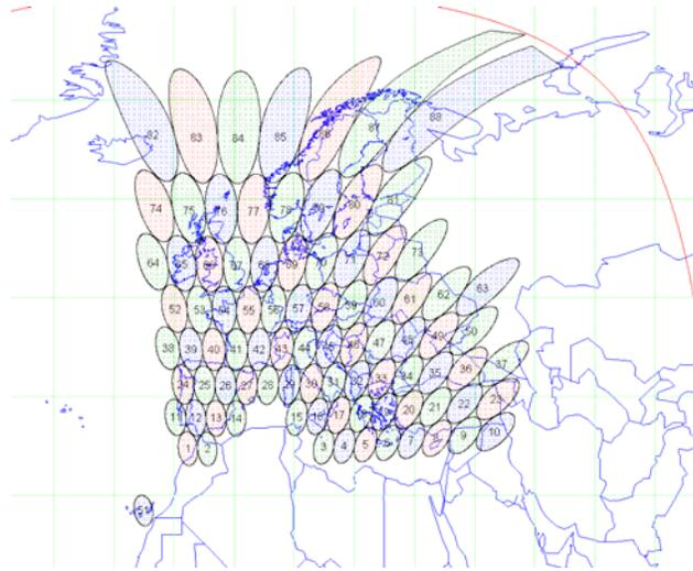
Figure 2. Representative 88 dual polarised user beams over Europe
