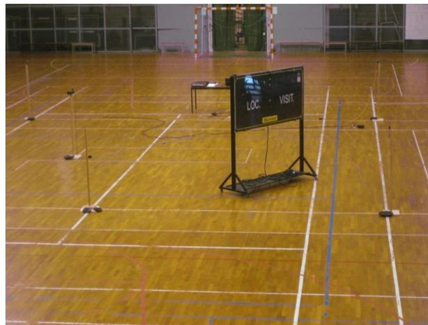
Figure 12. Metallic obstacle between the mobile transmitter and the receiving antenna 2.
