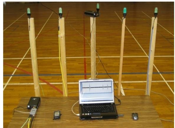
Figure 7. UWB TDOA localization experiment set-up.
