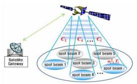
Figure 1. Multi-beam satellite system applying active beam selection scheme
