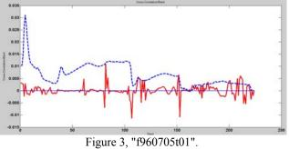
In Figure 3, Inter band Cross-correlation has been lost after the process of bit depth rescaling.
