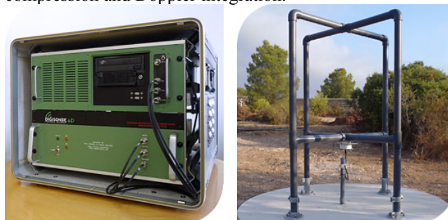
Figure 2. DPS-4 ionosonde and receive antenna
