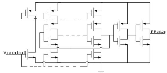
Figure 7. Voltage Controlled Oscillator
