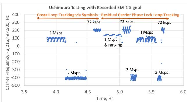
Figure 5. Uchinoura test with EM-1 signal, 2017-12-01
