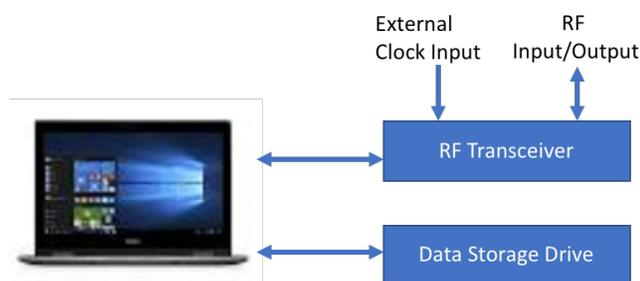
Figure 1. Components of the Recorder Playback Assembly
