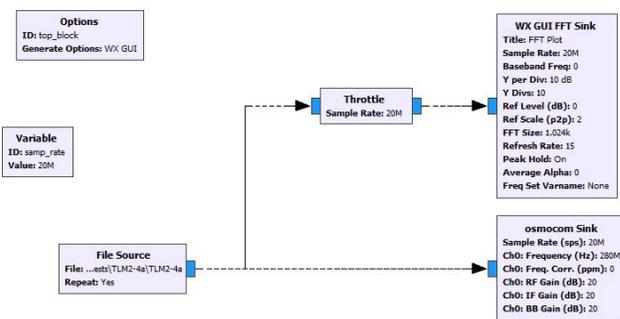
Figure 3. Control Interface for Playback
