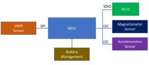
Figure 3. Overview of the device's architecture.
