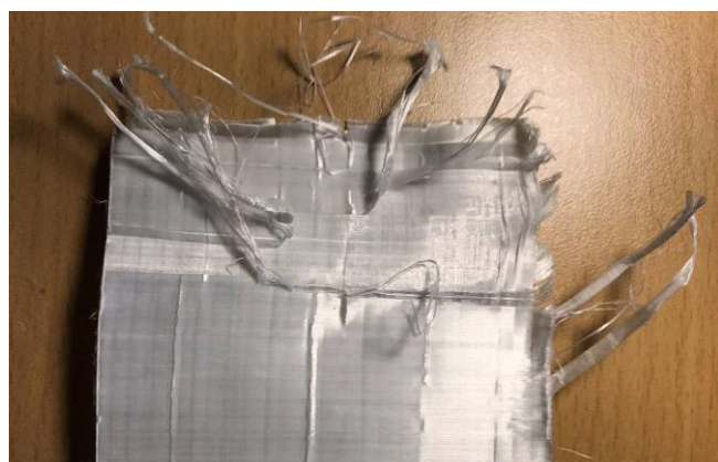
Figure 5. Damaged Dyneema® HB26 tape. Layer-, matrix- and bidirectional fiber structure is visible.
