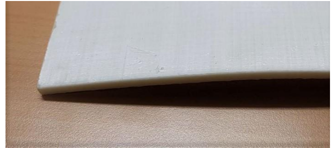
Figure 7. Hardened 20 layers Dyneema® HB26 plate after post-processing.
