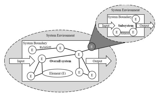
Figure 3: Structural modeling of a production system [12].
