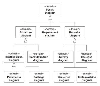
Figure 5: SysML diagrams according to [21].
