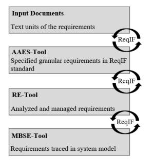
Figure 10: Process of requirements work from text to system model according to [34].
