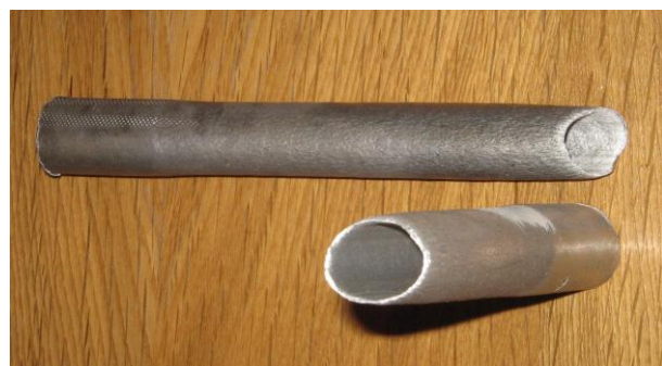
Figure 10. Broken aluminium pipe at maximum mechanical stretch [17].
