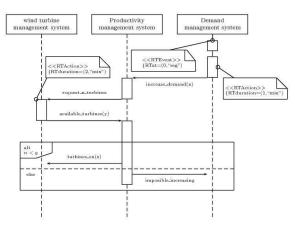
Fig. 3. Wind Turbine Management System Sequence Diagram
