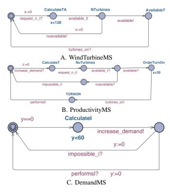
Fig. 4. Wind Mill Management System modeled in UppAal
