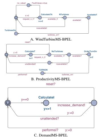
Fig. 5. Wind Mill Management System modeled in UppAal - from BPEL
