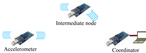
Figure 10. A network scenario with two hops between the sensor node and coordinator.
