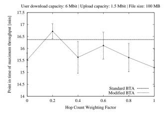
Figure 9. Point in time of maximum throughput for varying WF values. The result for standard BT is independent from WF values and therefore constant.
