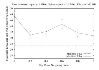
Figure 8. Maximum throughput in the whole network for varying WF values. The result for standard BT is independent from WF values and therefore constant.
