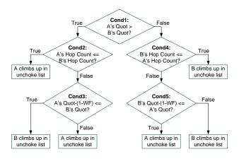
Figure 2. New BT choking algorithm for calculating a user's position in the unchoke list. The hop count is used as additional selection criterion.
