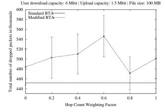
Figure 7. Number of dropped packets for varying WF values. The result for standard BT is independent from WF values and therefore constant.
