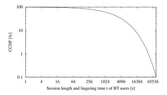
Figure 4. Complementary cumulative Weibull(t, 3302.977, 0.59) distribution function for the session length and lingering time of BT users. For the x-axis, a base 2 logarithmic scale is used; for the y-axis, a base 10 logarithmic scale is used.
