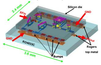
Figure 12. Top view of the simulated 4 GHz band-pass filter. Plastic of the package is not represented on the picture for clarity reason.
