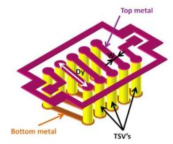
Figure 2. Synoptic representation of a 5 turns 3D solenoid within its RF test structure (bulk silicon is not represented on the picture)
