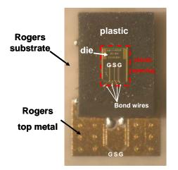
Figure 9. Photograph of the designed test-case suitable for microwave package characterization and modeling. Configuration allows 2 ports micro-probing: one on the inner die and the second one on the Rogers top metal (bottom of the picture)
