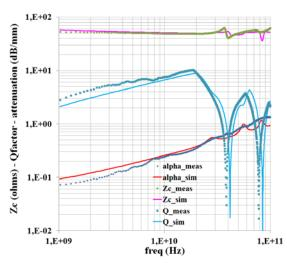
Figure 19. Comparison between measured and simulated data vs. frequency for transmission line characteristic impedance Zc, attenuation alpha and quality factor Q (length =  $2000 \ \mu m$ , width =  $15 \ \mu m$ , spacing =  $8.3 \ \mu m$ , 4 bends)
