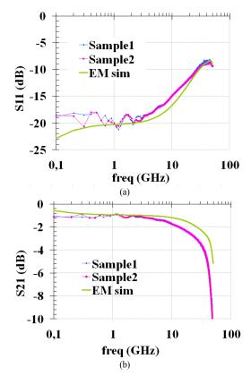
Figure 7. Comparison between Measured and simulated data on both (a) Reflection and (b) transmission S-parameter (1-turn solenoid)
