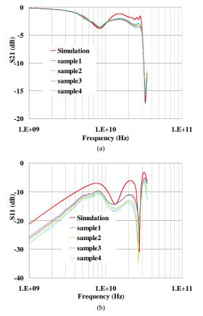
Figure 10. Comparison between measurements and simulated data vs. frequency on the package test-case – (a) transmission parameter, (b) reflection parameter
