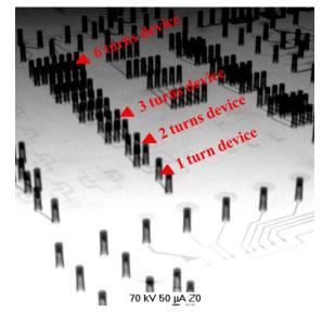
Figure 3. X-ray diffraction picture of the solenoid dedicated module (source IPDiA) – The bottom white face of the picture is the top side of the wafer
