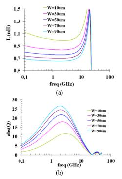
Figure 6. Simulated variations of (a) the self-inductance value and (b) quality factor vs. frequency for 1-turn solenoid (Dy was set to a fixed value during the simulations). These plots have been deduced from 2-ports Sparameter anlysis with a classical CAD simulator (i.e., SPICE). Compact model described in the previous paragraph has been used to extract the devices performances
