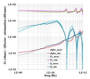
Figure 18. Comparison between measured and simulated data vs. frequency for transmission line characteristic impedance Zc, attenuation alpha and quality factor Q (length = 2000  $\mu$ m, width = 15  $\mu$ m, spacing = 8.3  $\mu$ m)
