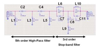
Figure 11. Schematic view of the 4 GHz band-pass filter considered for this study
