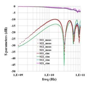
Figure 17. Comparison between simulated (EM) and measured Sparameter obtained on a transmission line (length = 2000  $\mu$ m, width = 15  $\mu$ m, spacing = 8.3  $\mu$ m)
