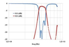
Figure 21. Simulated variations of transmission and reflection S-parameter of the proposed filter (nominal process parameters with copper back-end)
