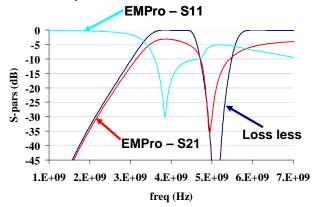
Figure 13. Simulation results of the proposed filter. Dark blue line corresponds to loss-less schematic filter simulated with ADS® schematic.
