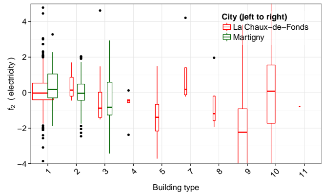
Figure 9. Discrepancy factor for the space heating, DHW and electricity services demands as a function of the building type in the version 3 simulations. Space heating and DHW show similar f_2 trends, as both are provided by the same ECS in most buildings. Allocation types: 1 apartment building, 2 individual home, 3 administrative, 4 schools, 5 sales, 6 catering, 7 meeting venues, 8 hospital, 9 industries, 10 warehouses, 11 sports installations, 12 indoor swimming pool.
