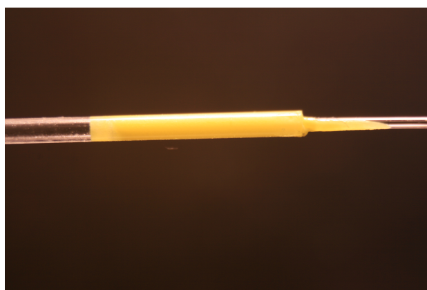
Figure 7. Optrode part where UV phosphor is deposited.
