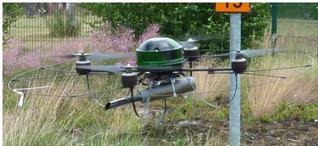
Figure 4. Micro-drone with multi-sensor equipment in flight.
