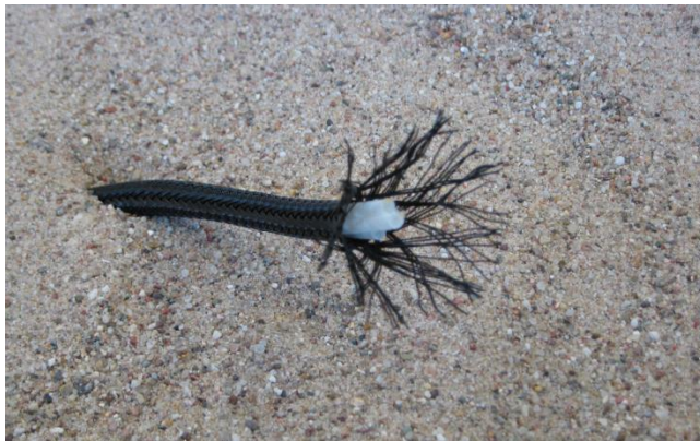
Figure 11. Membrane based gas sensor.
