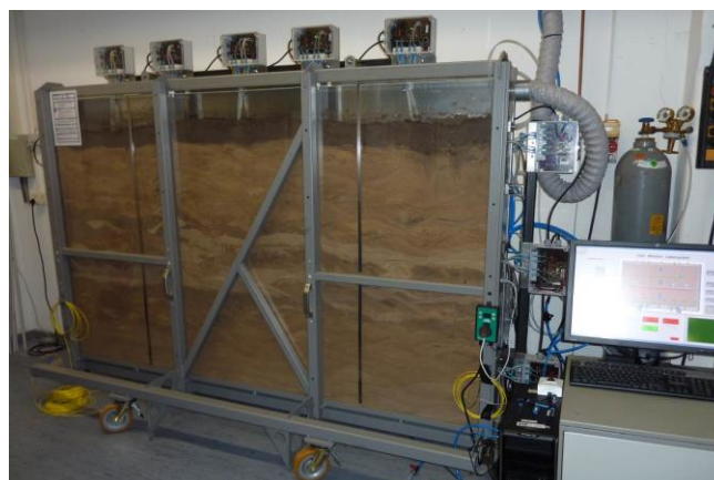
Figure 15. Laboratory setup with corresponding design to the test site and size of 2.5 x 1.5 x 0.1 m 3 .
