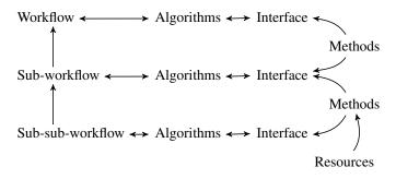
Figure 2. Workflow-algorithm sketch of a hierarchical implementation: Hierarchies of workflows, resources provided by methods.
