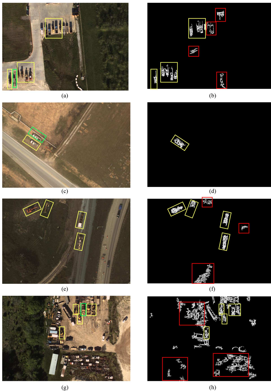
Figure 7. Results. Left column original RGB image. Right column – detection. Rectangles with yellow contours indicate true detections; rectangles with red contours - false alarms; rectangles with green contours - missed detections.
