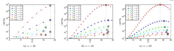
Figure 8. Normalized MTTDL declus vs. codeword length for  $s_{\rm eff}=1/2,2/3,3/4,4/5,5/6,6/7,$  and 7/8;  $\lambda/\mu=0.001$  and deterministic rebuild times.
