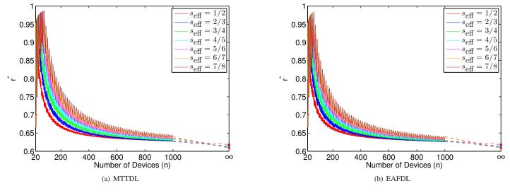
Figure 13.  $r^*$  vs. number of devices  $n \to \infty$ ,  $s_{\text{eff}} = 1/2, 2/3, 3/4, 4/5, 5/6, 6/7$ , and 7/8;  $\lambda/\mu = 0.001$  and deterministic rebuild times.
