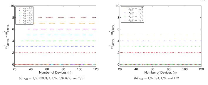
Figure 21. The difference between  $m^*_{\rm MTTDL}$  and  $m^*_{\rm EAFDL}$  vs. number of devices;  $\lambda/\mu=0.001$  and exponential rebuild times.
