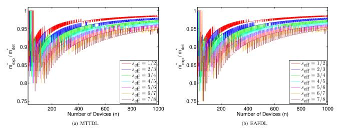
Figure 24. Ratio  $m_{\rm exp}^*$  to  $m_{\rm det}^*$  vs. number of devices for  $s_{\rm eff}=1/2,2/3,3/4,4/5,5/6,6/7,$  and  $7/8;\lambda/\mu=0.001.$
