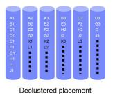
Figure 1. Clustered and declustered placement of codewords of length m=3 on n=6 devices. X1, X2, X3 represents a codeword (X = A, B, C, ..., L).
