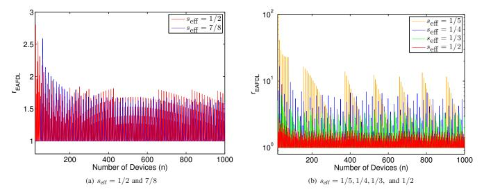
Figure 23. The EAFDL efficiency ratio  $r_{\rm EAFDL}$  vs. number of devices;  $\lambda/\mu=0.001$  and exponential rebuild times.
