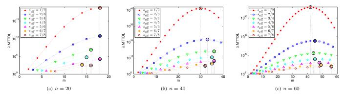
Figure 19. Normalized MTTDL declus vs. codeword length for  $s_{\rm eff}=1/2,2/3,3/4,4/5,5/6,6/7,$  and 7/8;  $\lambda/\mu=0.001$  and exponential rebuild times.
