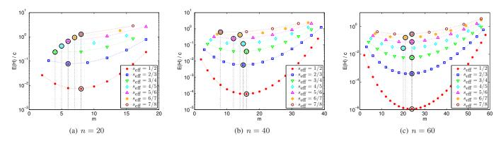
Figure 10. Normalized  $E(H)^{\text{declus}}$  vs. codeword length for  $s_{\text{eff}} = 1/2, 2/3, 3/4, 4/5, 5/6, 6/7$ , and 7/8;  $\lambda/\mu = 0.001$ .
