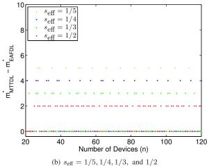
Figure 11. The difference between  $m_{\text{MTTDL}}^*$  and  $m_{\text{EAFDL}}^*$  vs. the number of devices;  $\lambda/\mu = 0.001$  and deterministic rebuild times.
