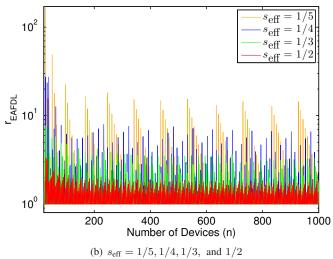
Figure 16. The EAFDL efficiency ratio  $r_{\text{EAFDL}}$  vs. number of devices;  $\lambda/\mu=0.001$  and deterministic rebuild times.
