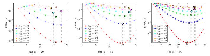
Figure 20. Normalized EAFDL declus vs. codeword length for  $s_{\rm eff}=1/2,2/3,3/4,4/5,5/6,6/7,$  and 7/8;  $\lambda/\mu=0.001$  and exponential rebuild times.
