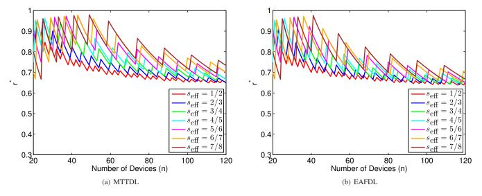
Figure 22.  $r^*$  vs. number of devices for  $s_{\rm eff}=1/2,2/3,3/4,4/5,5/6,6/7,$  and 7/8;  $\lambda/\mu=0.001$  and exponential rebuild times.
