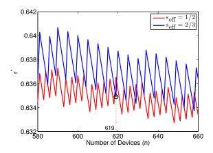
Figure 15.  $r^*$  for MTTDL vs. number of devices for  $s_{\rm eff}=1/2,2/3;$   $\lambda/\mu=0.001$  and deterministic rebuild times.
