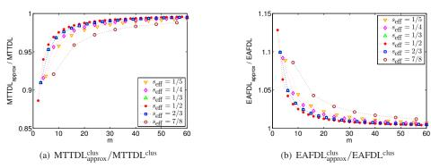
Figure 4. Accuracy of approximations for clustered placement vs. codeword length for  $s_{\rm eff}=1/5,1/4,1/3,1/2,2/3,$  and 7/8.
