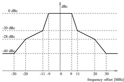
Figure 12: Spectral power mask of OFDM based WLAN.
