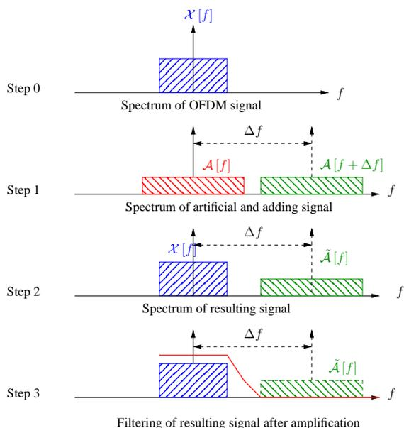
Figure 7: Mechanism of PAPR reduction.
