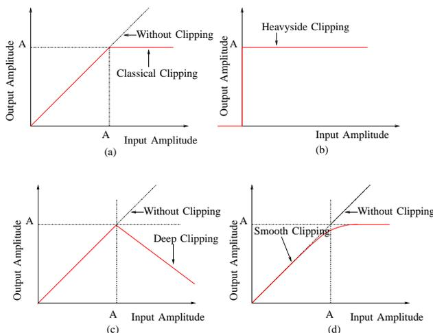
Figure 5: Functions-based clipping for PAPR reduction
