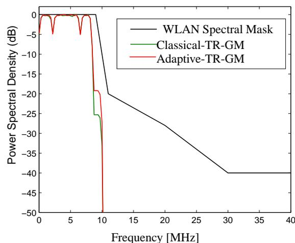
Figure 20: PSD of signals using "CT-MC" and "AT-MC" PAPR reduction technique ( $N_{iter} = 3$ ).
