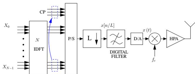
Figure 1: OFDM Transmitter Block Diagram.
