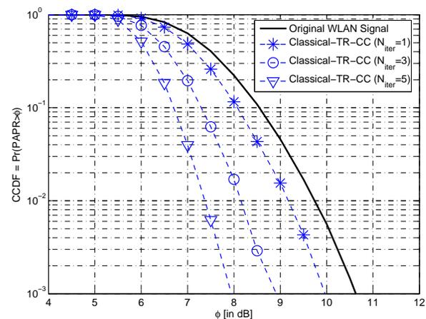
Figure 13: PAPR reduction performance for Classical-TR-CC technique for different iterations.
