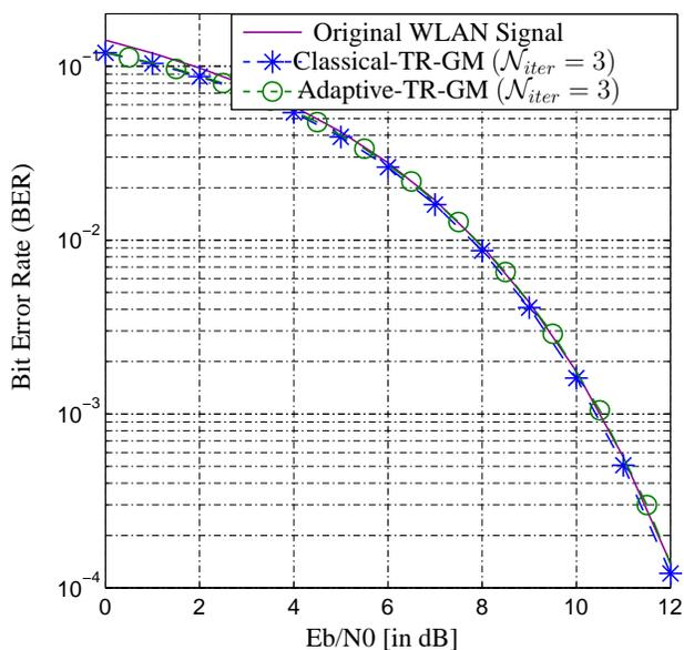
Figure 18: BER performance for Classical-TR-GM and Adaptive-TR-GM techniques over an AWGN channel.
