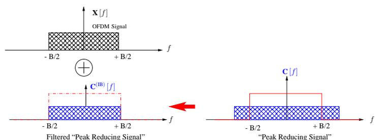
Figure 8: Out-of band distortion mitigation structure based on FFT/IFFT digital filter.
