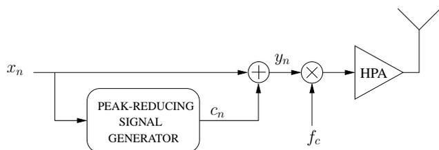
Figure 2: Adding Signal scheme for PAPR reduction.
