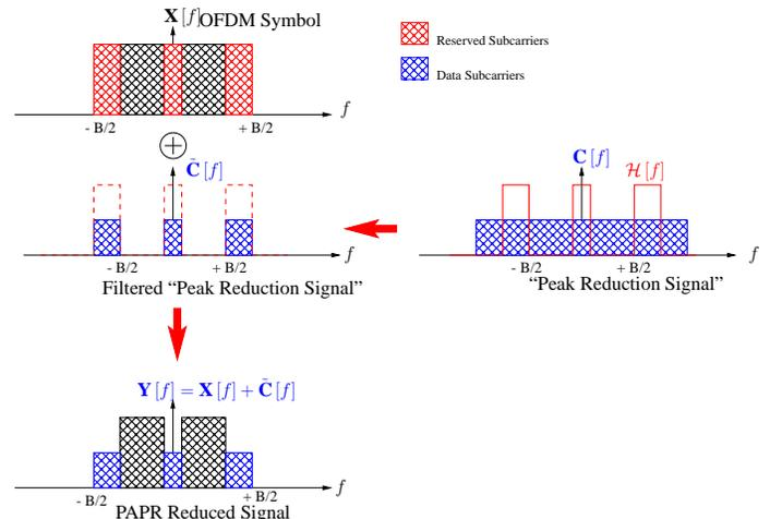
Figure 11: FFT/IFFT pair-based filter for transformation to TR technique.
