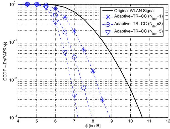
Figure 14: PAPR reduction performance for Adaptive-TR-CC technique for different iterations.
