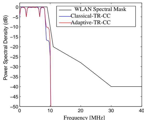
Figure 19: PSD of signals using "CT-CC" and "AT-CC" PAPR reduction technique ( $N_{iter} = 3$ ).
