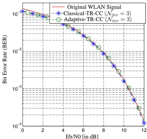
Figure 17: BER performance for Classical-TR-CC and Adaptive-TR-CC techniques over an AWGN channel.
