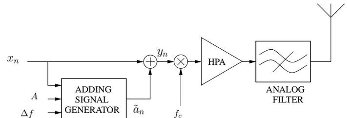
Figure 6: Principle of GM technique for OFDM PAPR reduction.
