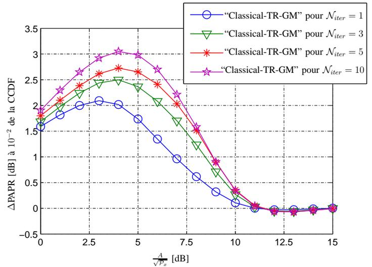
Figure 15: PAPR reduction performance of the Classical-TR-GM technique for different iterations number  $N_{iter}$ .
