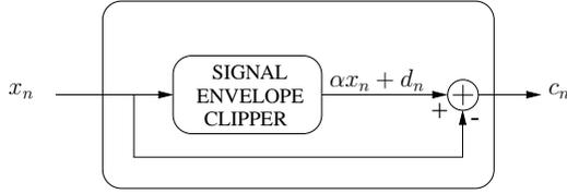
Figure 3: Peak-reducing signal generator block for clipping technique.
