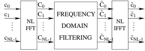
Figure 10: Digital filtering-based FFT/IFFT.
