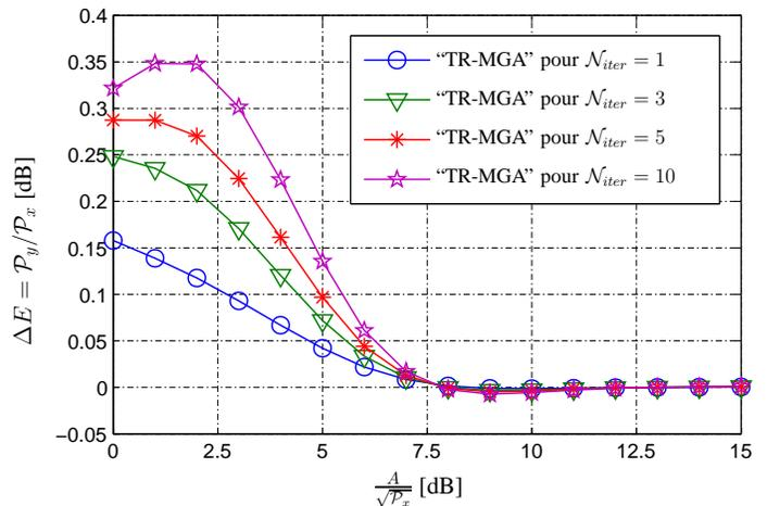
Figure 16: Average power ratio of the Classical-TR-GM technique for different iterations number  $N_{iter}$ .
