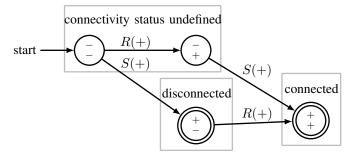
Figure 17: State Machine of Connectivity Status Calculation (S(+)) represents sender's sending notification, R(+) represents receiver's receiving notification)
