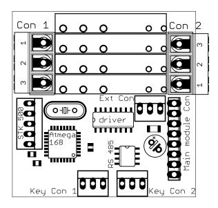
Figure 8. Execution module's PCB with connectors
