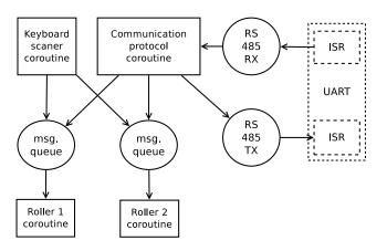
Figure 12. Architecture of executing module firmware
