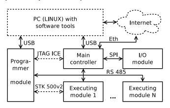
Figure 1. Modular schematic of the platform's hardware
