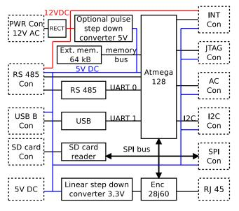
Figure 3. Ideological schematic of the main controller
