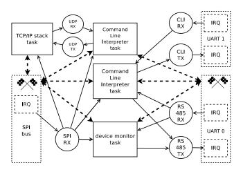
Figure 11. Architecture of main controller firmware
