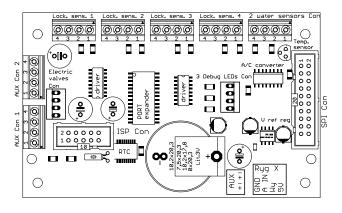
Figure 6. I/O module's PCB with connectors
