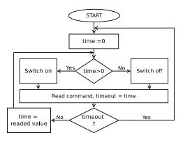
Figure 18. Algorithm for coroutine handling a single light source
