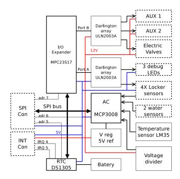
Figure 5. Ideological schematic (schematic diagram) of the I/O module
