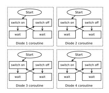
Figure 16. Algorithm for concurrent flashing of four light sources
