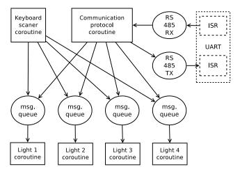
Figure 20. Architecture of executing module firmware controlling four light sources
