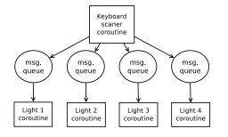
Figure 17. Architecture of executing module firmware controlling four light sources with keyboard
