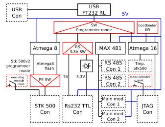
Figure 9. Ideological schematic of the programmer
