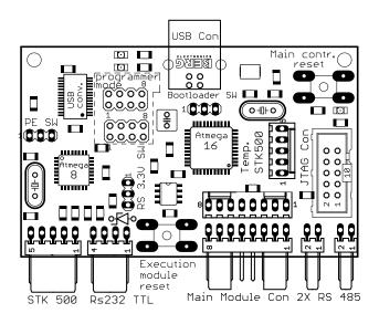
Figure 10. Programmer's PCB with connectors
