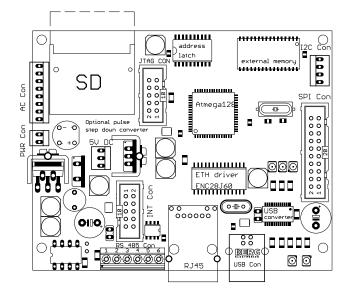
Figure 4. Main controller PCB with connectors
