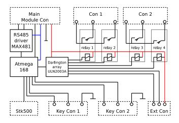
Figure 7. Ideological schematic of the executive module
