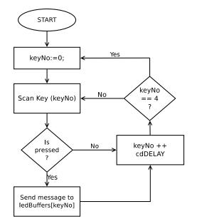
Figure 19. Algorithm for coroutine handling keyboard
