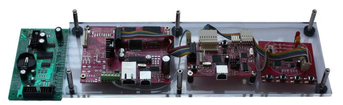
Figure 2. Didactic embedded platform: I/O module, main controller, programmer execution module.
