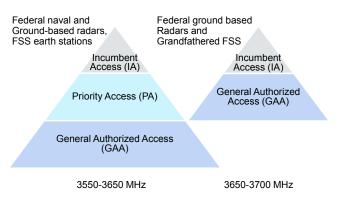
Figure 1. The US CBRS 3-tiered authorization framework with the FCC's spectrum access models for 3550-3650MHz and 3650-3700MHz spectrum segments.
