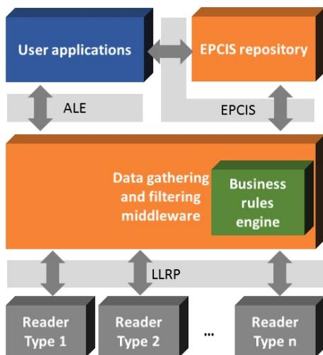
Figure 7. RFID management software architecture
