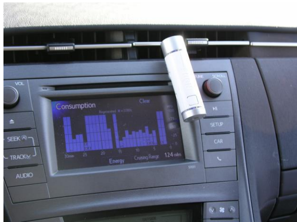
Figure 3. Personal mobile sensor mounted in a car near the vent.
