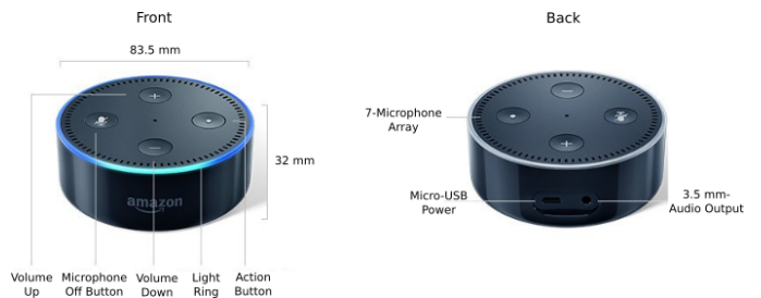
Figure 5. Basic structure of the Amazon Echo Dot [30]
