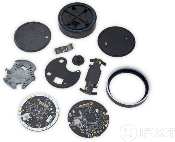
Figure 6. Teardown of the Echo Dot [5]
