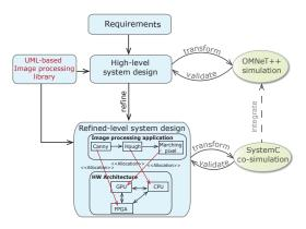
Figure 2: Design flow for image processing systems.
