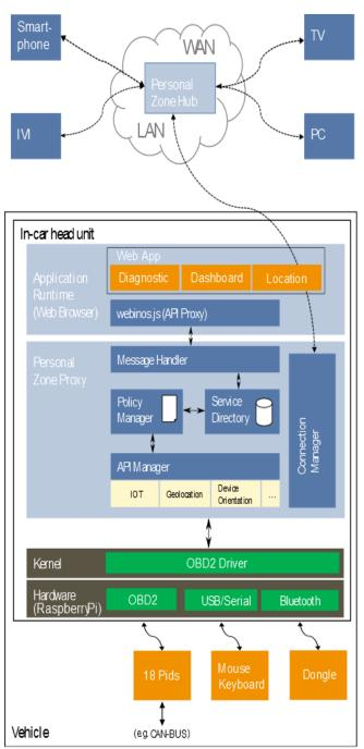
Figure 2: Architecture view how the *webinos* Middleware connects with OBD-II in a distributed automotive environment, similar to architecture [16]
