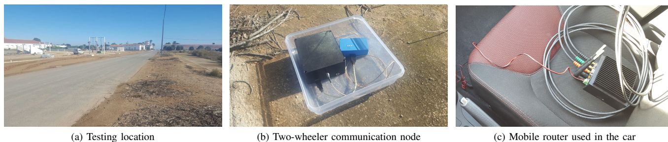
Figure 4. Scenario for testing one-hop communications using 802.11p
