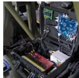
Figure 4. Electronic and communication control box
