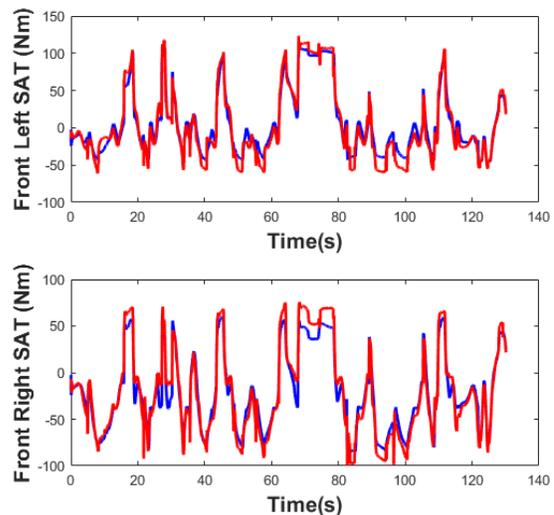
Fig. 6. Estimation results of SAT on wet asphalt; Blue (True) and Red (Estimated with NN).
