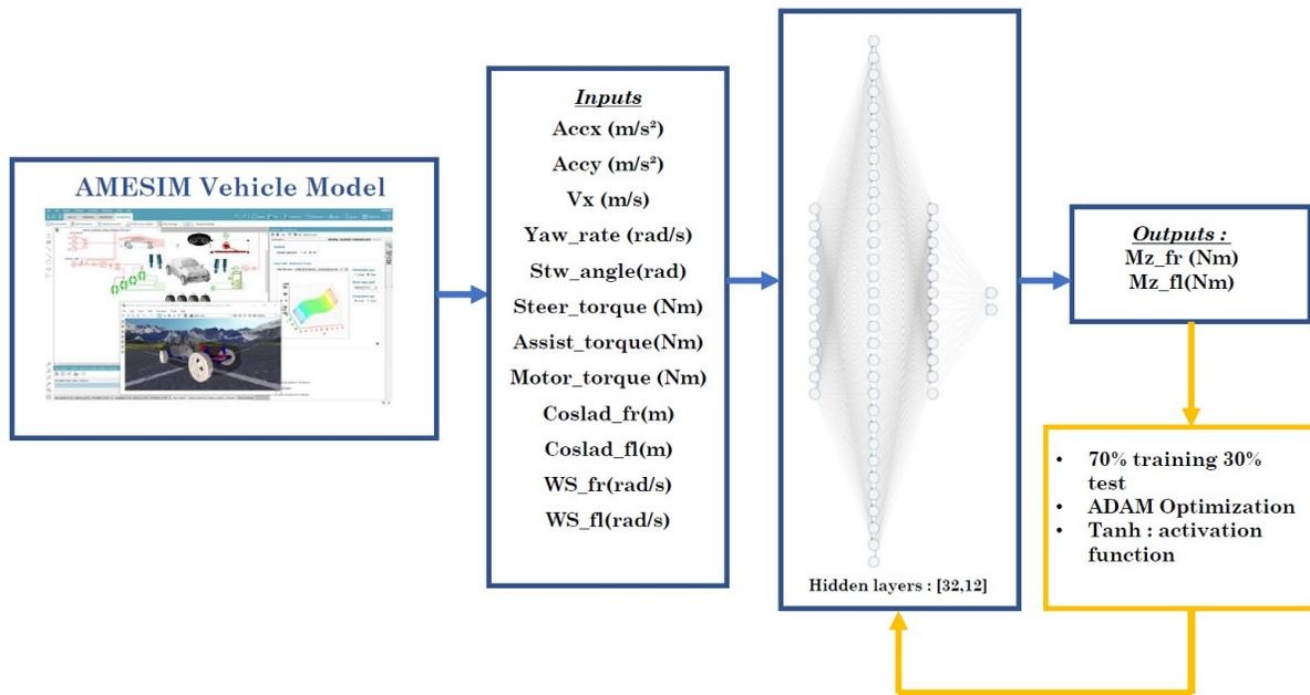
Fig. 3. SAT estimation structure, adapted from [8].
