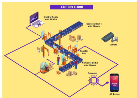
Figure 4: Proposed architecture solution for AR identification solution in Manufacturing Environment
