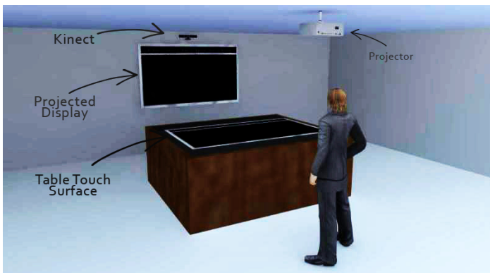
Figure 1. Extended wall and large touch surface system overview
