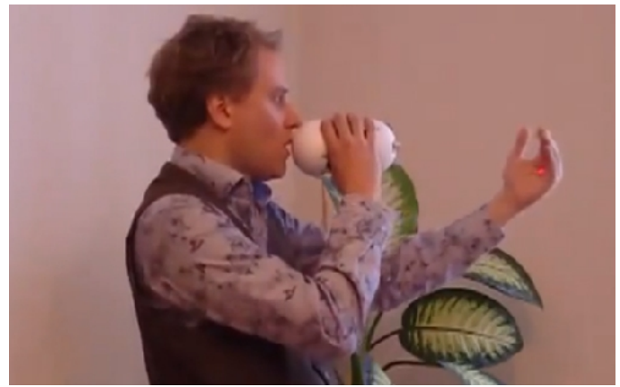
Figure 3: Playing the Trombosonic, the red laser in the palm indicates the direction of the ultrasonic sensor
