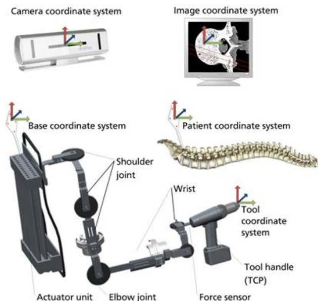
Figure 1 Overview of the robotic subsystem of the BOReScOPE.
