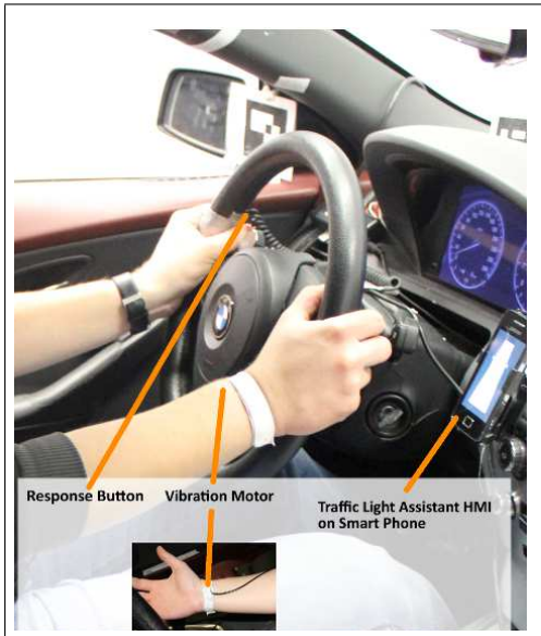
Figure 2. Setup of the devices in the driving simulator
