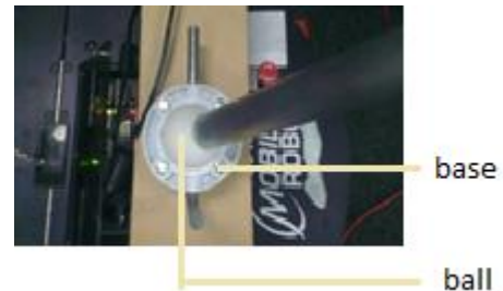
Figure 4. Ball-free mechanism at the Base.
