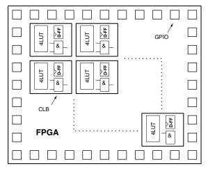
Figure 1. Simplified FPGA structure
