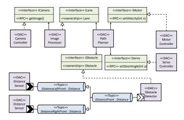
Figure 4. Example Architecture with communication paradigms
