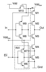
Figure 8. Low-power tristate buffer
