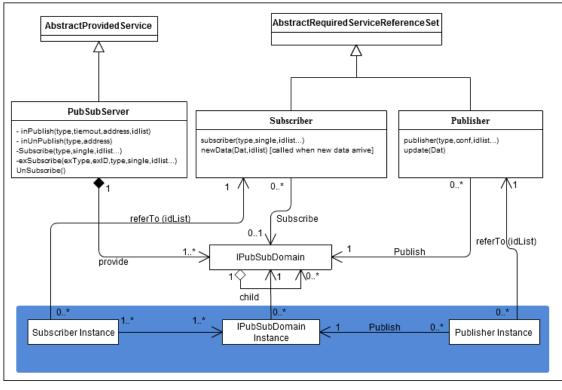
Figure 6. Core elements of the pub/sub system
