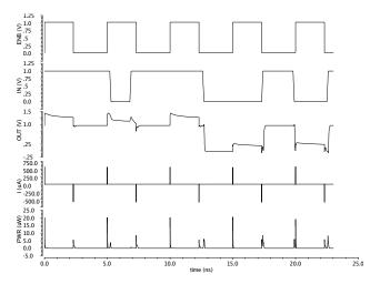
Figure 9. Simulation results of dynamic behavior of the low-power tristate buffer
