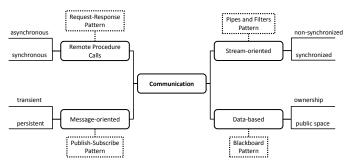
Figure 1. Adapted Communication Taxonomy for distributed Systems based on [22] and [23]
