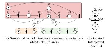
Figure 1. Dynamic control structures from [15]
