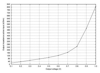
Figure 10. Output impedance in highZ state (low power tristate buffer)
