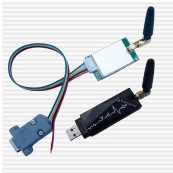
Figure 4. PLC Wi-Fi attachments (upper one for PLC, other one for PC)
