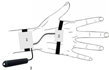
Figure 3. Schematic of the wearable motion-sensing prototype
