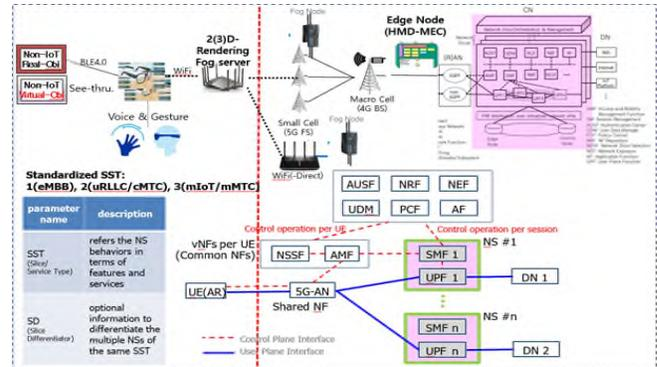
Figure 7. The DEC adapting to 5G Core Plane Prototype
