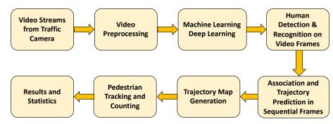
Figure 1. End-to-end system architecture.
