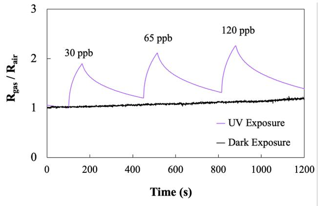
Figure 5. Ozone detection, at an operating temperature of 50°C, in dark and under UV illumination for a WO<sub>3</sub> film prepared with a 1:1 Ar/O<sub>2</sub> ratio.
