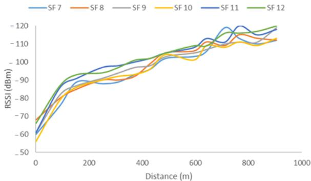
Figure 9. RSSI for 433 MHz and 5dBi antenna.
