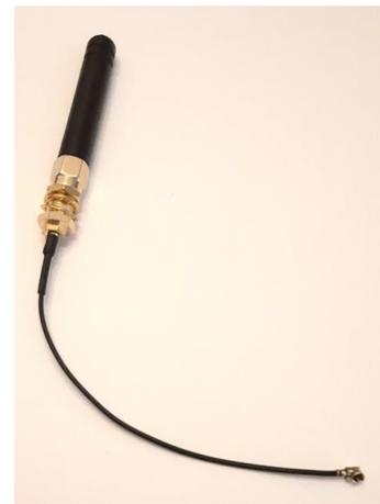
Figure 4. 868 MHz antenna.
