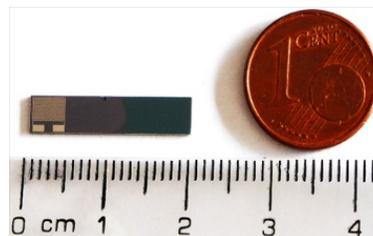
Figure 1. Sample image of SiO<sub>2</sub>/Si substrate (4 x 4 mm<sup>2</sup>) with platinum electrodes and a trioxide tungsten layer above it
