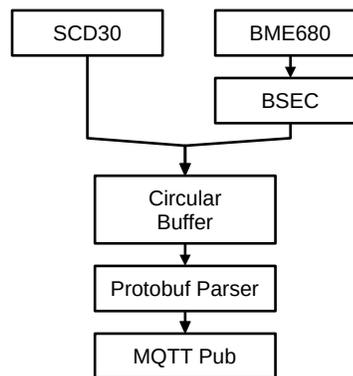
Fig. 2. Internal data flow of the sensor node
