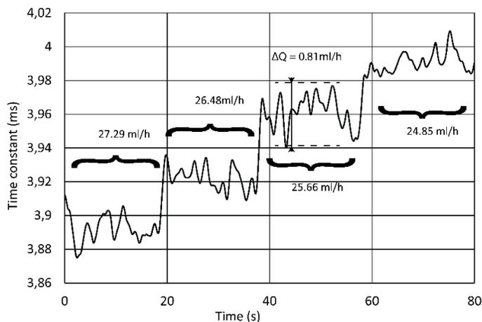
Figure 7. Demonstration of sensor resolution and time response at low flow rates
