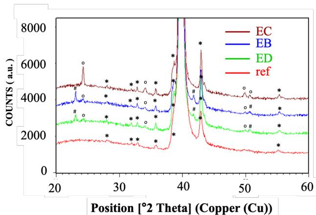
Figure 3. Comparison of WO<sub>3</sub> diffractograms with reference test platform (\*) using  $\lambda = 1.54\text{\AA}$  (Philip's X'Pert MRD).
