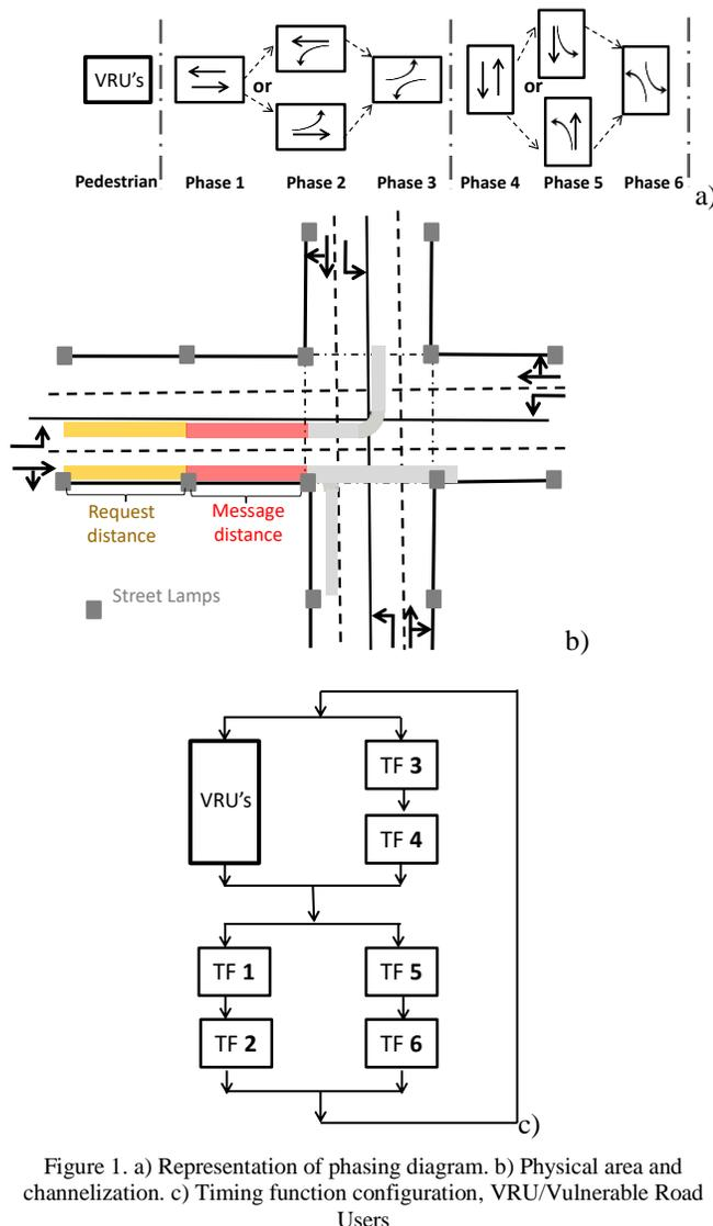
Figure 1. a) Representation of phasing diagram. b) Physical area and channelization. c) Timing function configuration, VRU/Vulnerable Road Users
