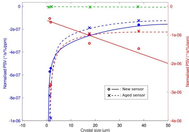
Figure 5. Phase shift velocity normalized by surface coverage and gas concentration measured under CO<sub>2</sub>, CO and O<sub>2</sub>.
