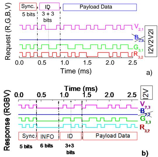
Figure 3. Frame structure representations. a) Codification used to drive the headlights of a vehicle in a request message from footprint #8.  $R_{3,2}$ ,  $G_{3,1}$ , and  $V_{2,1}$  are the transmitted node packet, in a time slot .b) Encoded message response of the controller to the request message of the vehicle in position #8 ( $R_{3,2}$ ,  $G_{3,1}$ , and  $V_{2,1}$ ).
