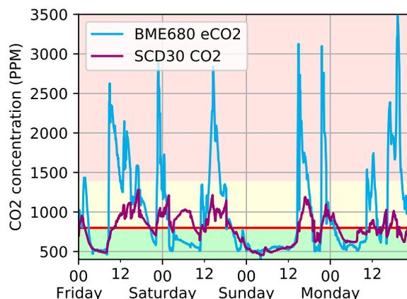
Fig. 4. Recorded actual (SCD30) and VOC based estimated (BME680) CO<sub>2</sub> concentration
