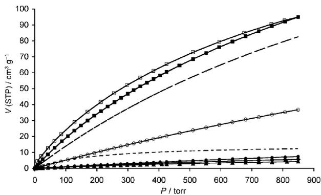
Figure 4. SEM Adsorption-desorption isotherms for ZnTACN MOF at 298 K with CO<sub>2</sub> (ads: ■, des: □), CH<sub>2</sub> (○), CO (●), N<sub>2</sub> (◆), and O<sub>2</sub> (▲).
