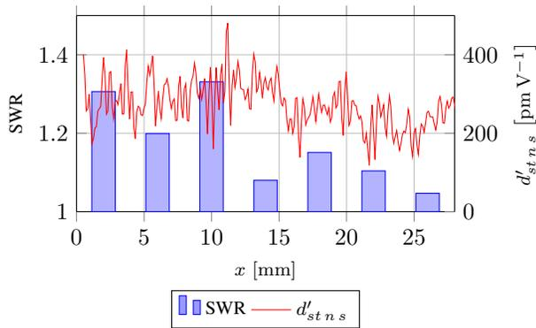
Fig. 10. Measured standing wave ratio (SWR) and relative amplitude  $d'_{st,ns}$  of normal displacement of substrate surface along SAW traveling direction for SAW motor with non-piezoelectric stator material; SWR was sectionally determined by method of least squares
