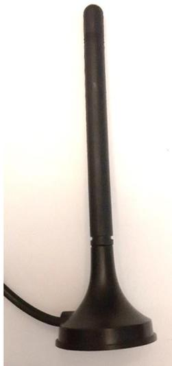
Figure 2. 433 MHz antenna with a gain of 3dBi.
