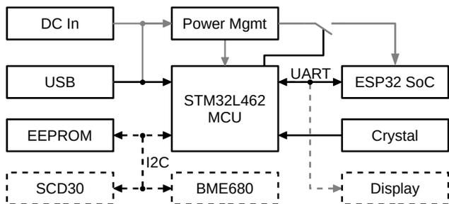
Fig. 1. Hardware block diagram of the sensor node
