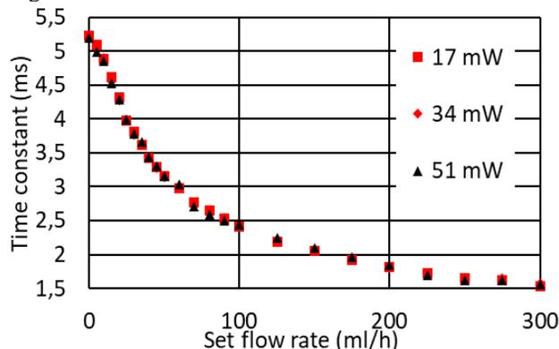
Figure 6. Dependency of measured result from heating power
