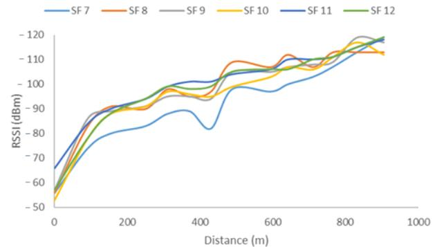
Figure 8. RSSI for 433 MHz and 3dBi antenna.
