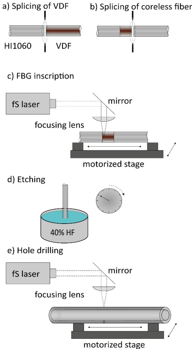
Figure 3. Manufacturing procedure
