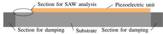
Fig. 4. Basic structure of transient FEM model
