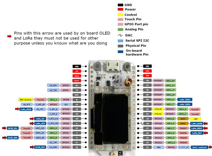
Figure 6. Heltec Wi-Fi 32 LoRa module pinout.
