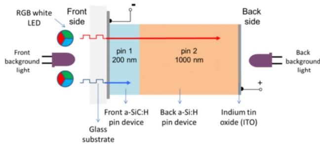
Figure 3. Simplified cross-section view of the photodetector.
