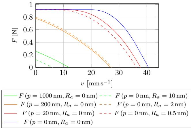
Fig. 7. Motor characteristics by motor model depending on varying spherical elevations  $p$  and average roughness values  $R_a$ ; Motor as described in [7] with a normal SAW amplitude of 3 nm at the surface and an overall contact force of 4 N
