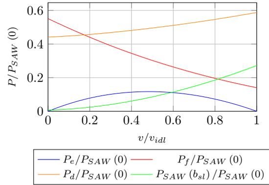
Fig. 8. Calculated effective power  $P_e$ , friction losses  $P_f$ , dynamic losses  $P_d$  and remaining SAW power  $P_{SAW}$  behind the slider for a SAW motor as described in [14]; Total contact force  $F_N = 80$  N; Assumed roughness  $R_a = 1$  nm due to used thin-film technology
