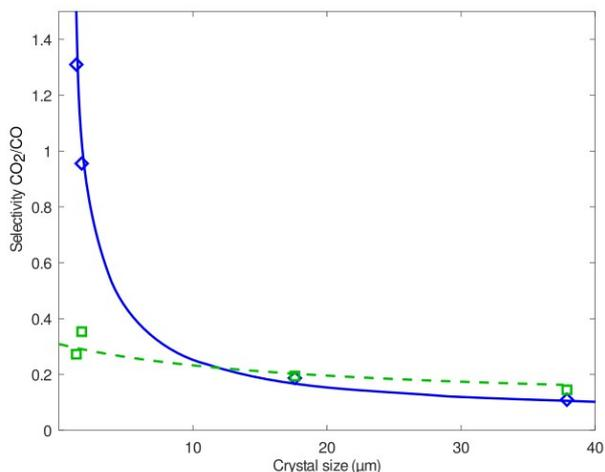
Figure 6. Selectivity CO<sub>2</sub>/CO versus MOF crystal size for new sensors and aged sensors.
