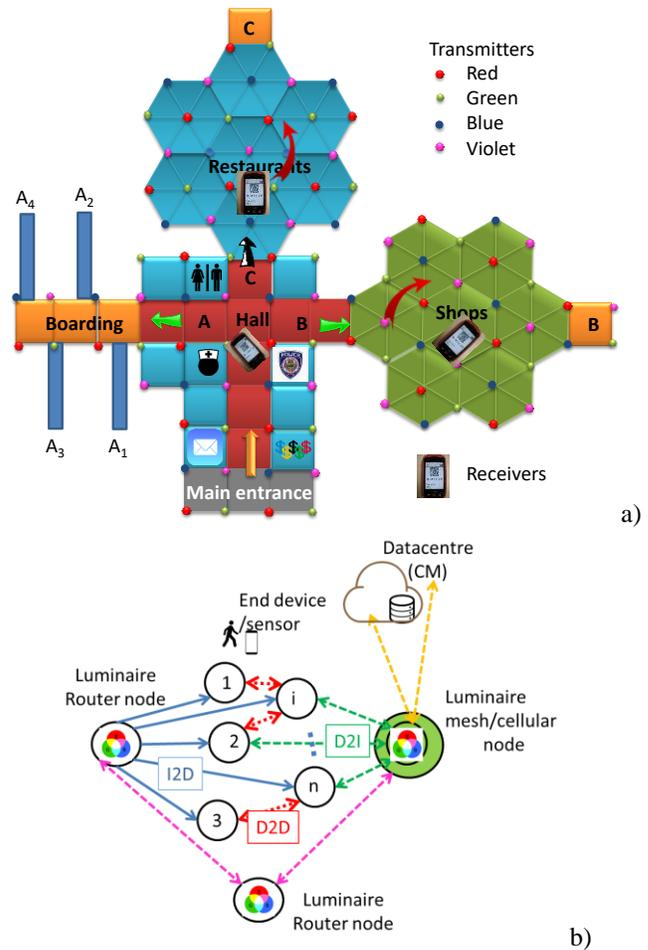
Figure 1 a) Optical infrastructure and indoor layout. b) a) Mesh and cellular hybrid architecture
