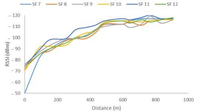
Figure 7. RSSI for 868 MHz and 3dBi antenna.
