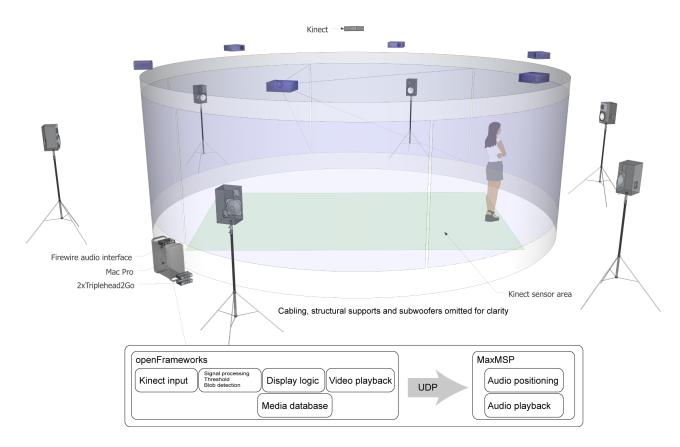
Figure 7. Diagram showing layout and main hardware and software components.
