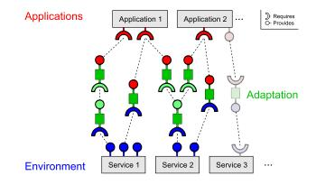
Figure 1. Proposed EAA architecture – *Environment* provides low-level services. *Applications* manipulate only high-level abstract services. *Adaptation* bridges the two and is dynamically extensible and user-controlled. Lighter chain on the right: inversion due to the whiteboard pattern.
