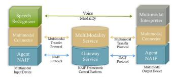
Figure 2: Software stack of an exchange of voice modality between a speech recognizer system as input and a published multimodal output system.
