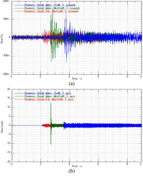
Figure 10. Measured (a) reflection sound pressure and (b) shock acceleration.
