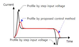
Figure 2. DC motor control method having soft-start and soft-stop current profile.
