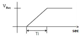
Figure 3. Applying voltage to DC motor for the generation of the softstart current profile.
