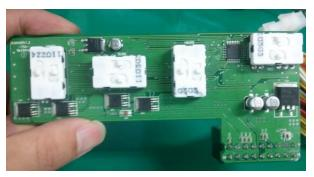
Figure 5. Developed DC motor driver having the functions of soft-start and soft-stop.
