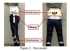
Motors with encoders were positioned on the axis of the hip joints for the purpose of measuring hip joint angles. Two potentiometers were positioned on the axis of the ankle joints for the purpose of measuring hip joint angles. An
