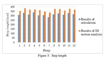
Figure 5 shows that the measurement error is 2.57(%) and standard deviation is 1.54(mm). The method that proposed had limitation of measurement accuracy. However, the results of calculation could be corrected by using the decided correction coefficient because standard deviation is very small.
