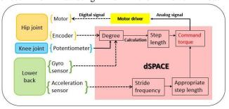
Figure 4. Real-time control system using dSPACE
