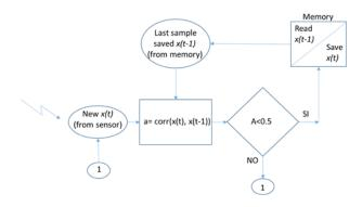
Figure 3. Monitoring process algorithm
