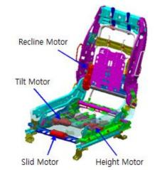
Figure 1. Configuratin of power seat having recline motor, tilt motor, slide motor, and height motor.
