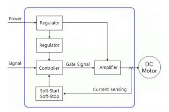
Figure 4. Control block diagram of DC motor driver.
