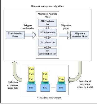
Figure 2. Multi-tier architecture of vGreen system.
