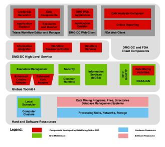
Figure 1. The DMG-DC architecture
