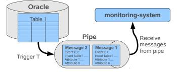
Figure 4. Monitoring using Triggers and Pipes
