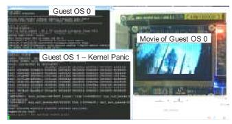
Figure 8. Virtual Machine Isolation
