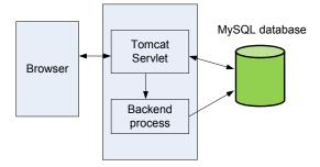
Figure 3. CCV implementation architecture.
