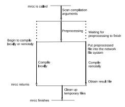
Figure 2. The work flow of mrcc
