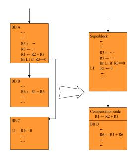
Figure 4. Build superblock based on profiling.
