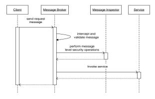
Figure 4. UML sequence diagram - Message Broker component
