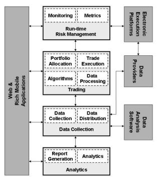
Figure 1. Reference component architecture of a contemporary onpremise high-frequency trading platform.
