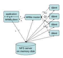
Figure 3. The architecture of MRlite
