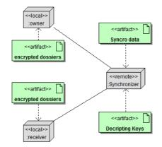
Figure 3. Deployment diagram of multi-agent system
