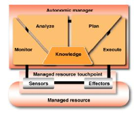
Figure 1. Autonomic loop (or MAPE/MAPE-K loop) [1].
