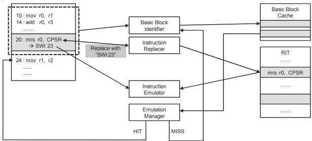
Figure 3. CPU Virtualization Architecture
