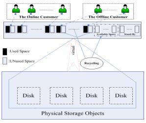
Figure 5. The Space Recycling Mechanism
