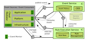
Figure 2. The Components of the Activity Service
