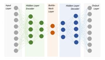
Figure 6. Basic Architecture of a Deep Autoencoder
