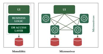
Fig. 1. Architecture of Monolithic and Microservices. Monothilic application blocks are defined and deployed as single units. Microservices offer more flexibility by decoupling an application into several small units and deploying independently.
