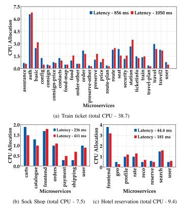
Fig. 2. Impact of resource distribution among microservice in response time. The X-axis shows the microservices in each applications, and the Y-axis shows the CPU allocation of each microservices.
