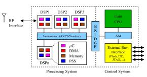
Fig. 1. The architecture of an Embb instance
