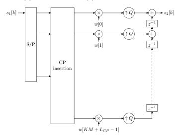
Figure 2. Transmitter of the windowed CP-FBMC/COQAM system.
