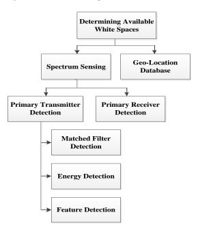
Fig. 5. Methods used for white spaces determination.
