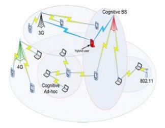
Fig. 3. CRNs operate inside the coverage area of primary networks [12].
