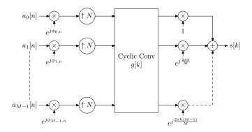
Figure 1. FBMC/COQAM baseband modulation.
