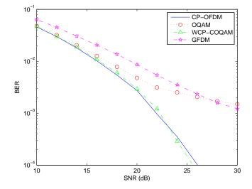
Figure 6. BER for uncoded QPSK in dispersive channel with ZF equalizer.
