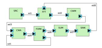
Fig. 6. WPD waveform DataFlow Graph of level L1
