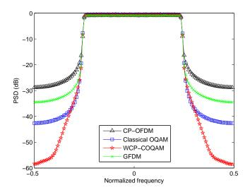
Figure 3. PSD simulation, M = 128, SRRC with roll-off 0.5.
