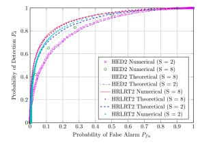
Theoretical and numerical ROC plot of hybrid approach 2 of Fig. 4. ED/RLRT. Parameters: N = 80, M = 80, K = 4 and SNR = -10dB
