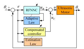
Figure 1. The proposed control scheme for the USM.
