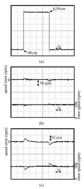
Figure 10. The experimental results for the USM rotor speed command of 100 rpm with 0.5N-m load. (a) applied load, (b) rotor speed and speed error using the proposed control scheme, (c) rotor speed and speed error using the PI control.
