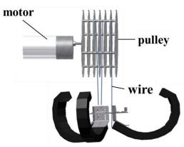
Figure 7. Mechanism to move the arms.
