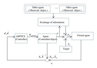
Figure 1. Structure of the proposed multi agent control system.
