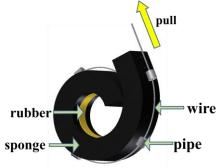
Figure 4. Structure of an arm.
