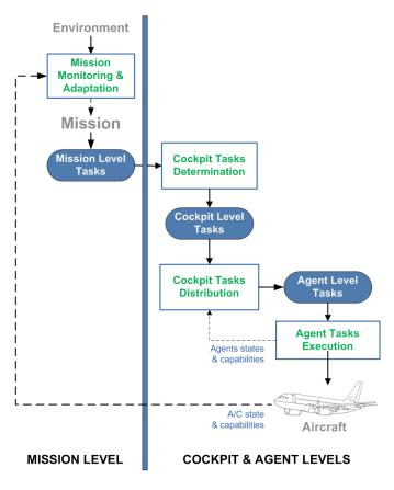
Figure 3. General Architecture for Adaptive Human-Automation Cooperation.
