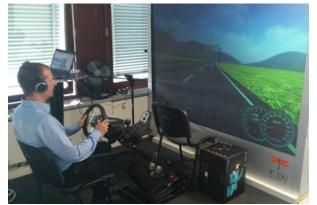
Figure 2. Driving simulator setup.
