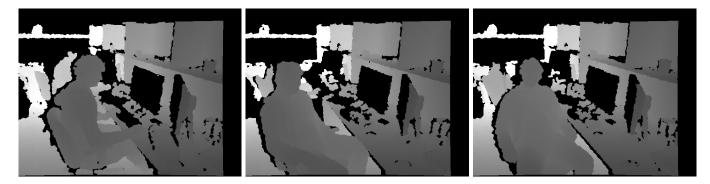
Figure 2. Representative raw-depth images of the three levels of attention. From left to right, *null* attention, *partial* attention and *full* attention. The images were captured using a Kinect<sup>TM</sup> mounted on the PR2 head.
