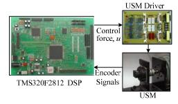
Figure 3. The USM experiment setup.
