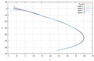
Figure 5. Trajectories of all the agents using LSM (  $\gamma = 0$  in (18)).
