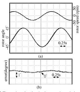
Figure 7. The experimental results using the proposed control scheme for a sinusoidal command from -45 to 45 degree. (a)USM rotor angle and speed responses, (b) angle error.
