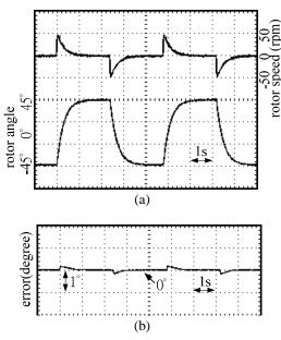
Figure 4. The experimental results using the proposed control scheme for a periodic square command from -45 to 45 degree. (a)USM rotor angle and speed responses, (b) angle error.
