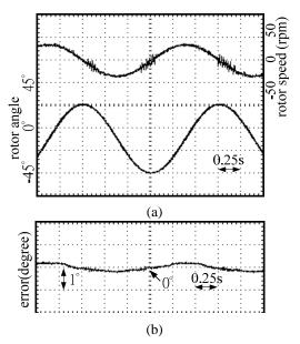
Figure 8. The experimental results using the RFNNC without compensated controller for a sinusoidal command from -45 to 45 degree. (a) USM rotor angle and speed responses, (b) angle error.
