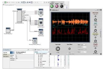
Figure 4. RTMaps for audio feature extraction.
