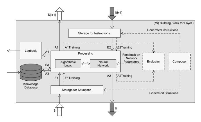
Fig. 2. Pattern of building block that implements each layer.
