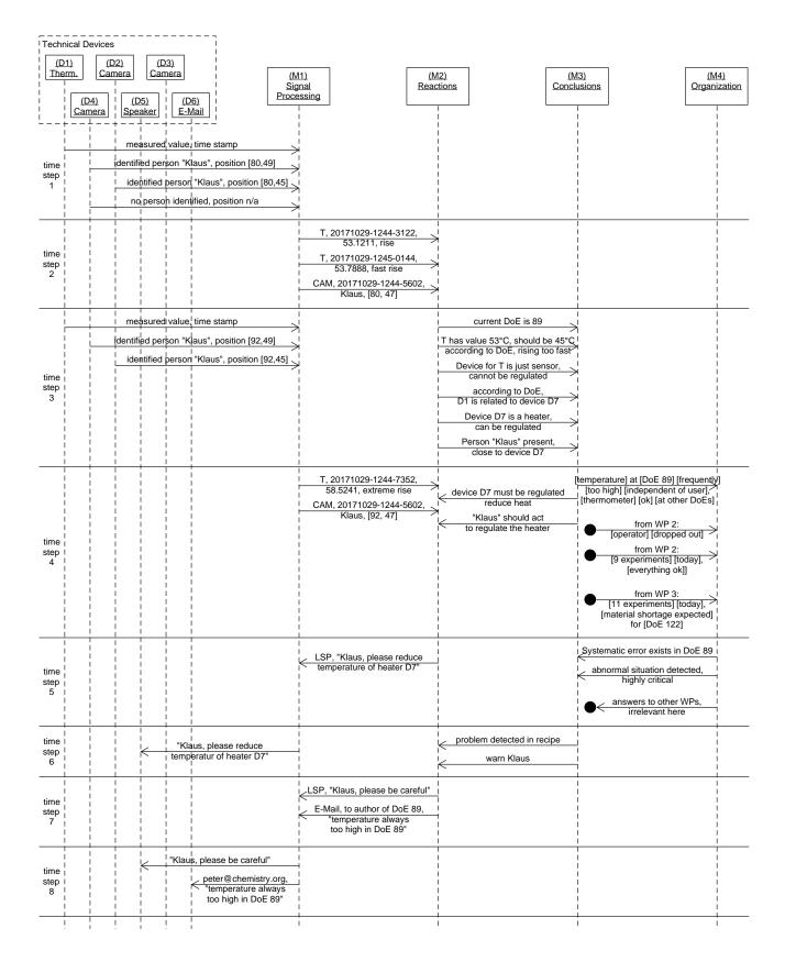
Fig. 4. Information flows between processing layers, for an exemplary execution of the system.
