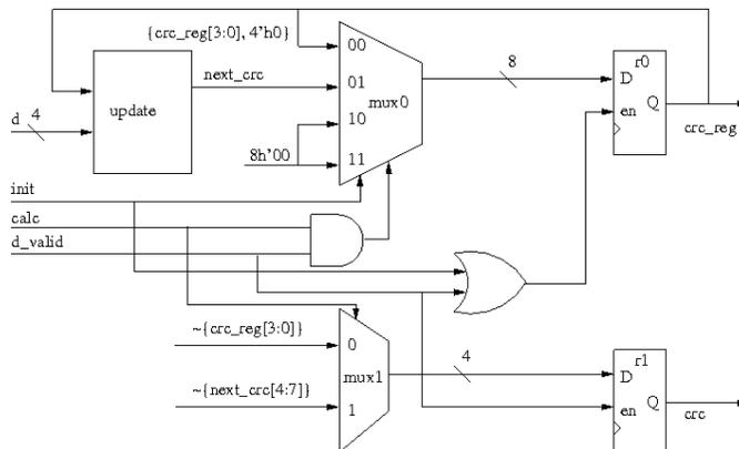
Fig. 6. A circuit to generate CRC code (adapted from [15]).
