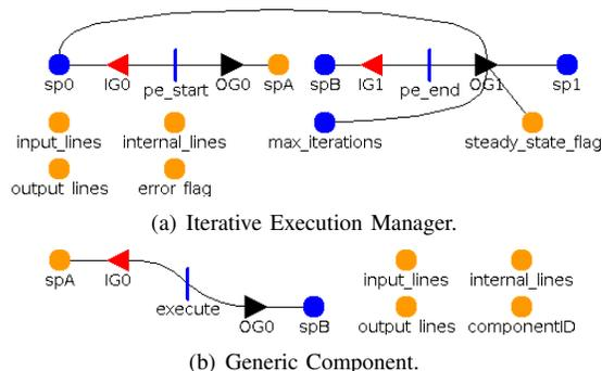
Fig. 4. Sub-modules of the Combinatorial and Sequential Logic SAN model.
