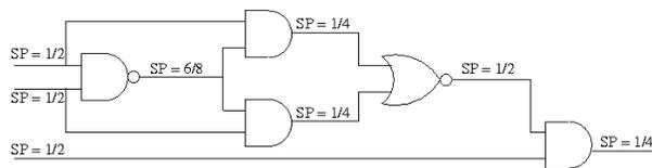
Fig. 5. Example of combinatorial circuit used for validation.
