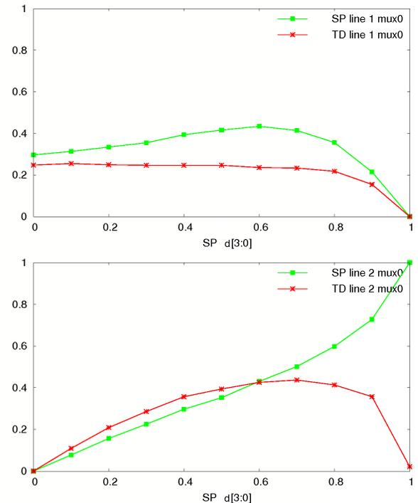
Fig. 7. Example of results for signal probability and transition density of two input lines of `mux0` for input data signal probability 0.5.
