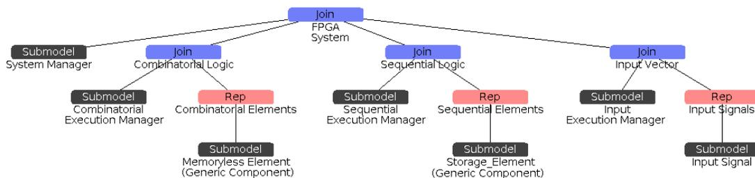
Fig. 1. SAN model of the FPGA.
