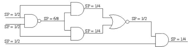
Fig. 5. Example of combinatorial circuit used for validation.
